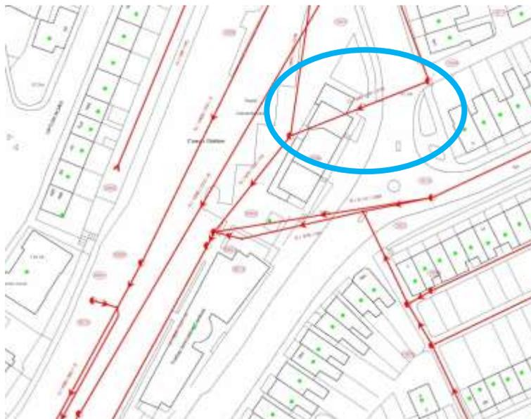
*Plan showing mains sewer to be relocated*
